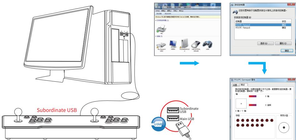
Open the device and printer, select the gamepad option, right click, select the game controller settings, enter the handle test interface.
